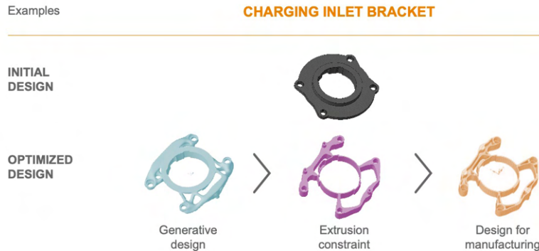
Figure 5 — Product designs can be iterated using state-of-the-art simulation techniques combined with artificial intelligence. The optimal shapes found can reduce the amount of material needed to fulfill all specifications and manufacturing constraints.
